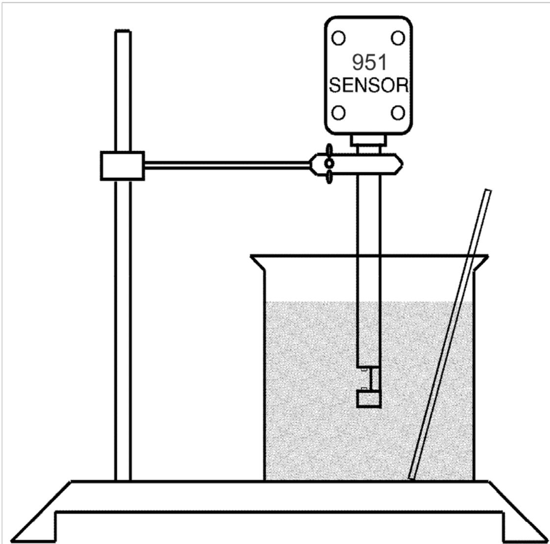
The calibration is a two-step procedure. Samples at each end of the desired range should be available.
