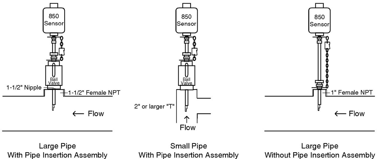
**Transparent Lines:** If the sensor is to be used in a transparent (e.g., glass, PVC, acrylic, etc.) process or sample line, the pipe must be wrapped with tape to prevent ambient light from entering the pipe and affecting the readings. Wrap the pipe five (5) pipe diameters from the sensor. **Black PVC electrical tape will not block light sufficiently.** Use an aluminum tape or wrap any tape over a metallic foil.
