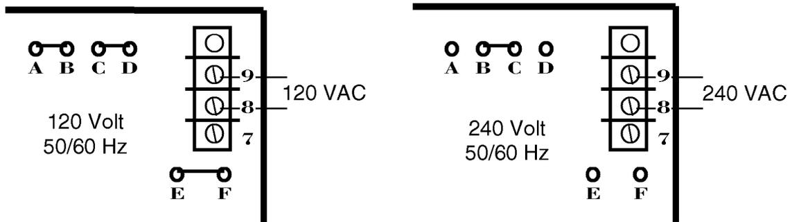
**DC Power Connections:** For 12V or 24V DC-powered operation, make all connections as above except for power connections. Connect **DC Positive (+) to terminal 9** and **DC Negative (-) to terminal 8**. The jumpers are factory set and do not need adjustment. Be sure that there is a good **earth-ground to terminal 7**.
