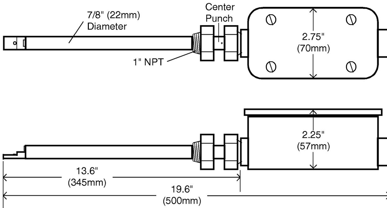
**Line Size:** There are no restrictions on the maximum pipe diameter into which the sensor can be installed. However, if a 2-inch or smaller line is to be monitored, install a 2-inch or larger "T" to prevent the sensor from blocking the line (see Figure C on page 3 for drawings of typical installations).
